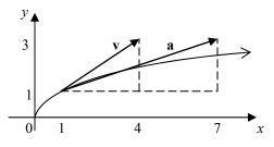
Example 2 Find the velocity, acceleration and speed of a particle whose position vector is given by  $\mathbf{r}(t) = e^t \mathbf{i} + e^{-t} \mathbf{j}$ ,  $t \ge 0$ . Sketch the path of the particle and draw the velocity and acceleration vectors at t = 0.
