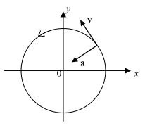
Example 4 An object moves in a path with position vector  $\mathbf{r}(t) = \cos t \mathbf{i} + 2\sin t \mathbf{j}, t \ge 0$ . (a) Show that the path is elliptical. (b) Show that the acceleration points towards the origin.
