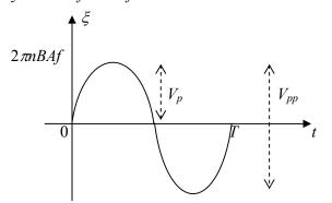
The amplitude of the sinusoidal voltage is called the peak voltage  $V_{p}$ ,
