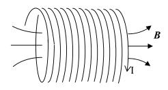
The magnetic field inside the solenoid is uniform.
