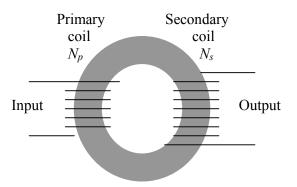
The primary (input) winding, of  $N_p$  turns, is connected to an alternating emf generator. The secondary (output) winding, of  $N_s$  turns, is connected to a load resistance *R*.
