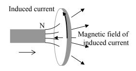
Magnetic field increases as the magnet moves towards the loop resulting in more flux to the right through the loop. The induced current *opposes* the flux increase by generating magnetic field to the left inside the loop. To achieve this the induced current flows anticlockwise (view from the magnet side).
