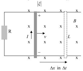
Electrical energy dissipated in R = Work done by the applied force.
