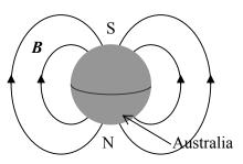
By convention, magnetic field lines always point away from N, the **north magnetic pole**, towards S, the **south magnetic pole**. The north magnetic pole (sometimes called the north seeking pole) of a compass points in the same direction as the magnetic field lines. A stronger magnetic field is indicated by closer magnetic field lines. The lines do not cross each other because the magnetic field cannot be pointing in more than one direction at any location.
