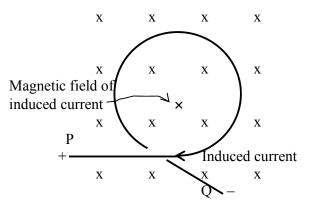
When the enclosed area decreases the magnetic flux through the loop into the page decreases. According to Lenz's law, the induced current generates magnetic field (hence flux) through the loop into the page to make up for (to *oppose*) the decrease in flux. To achieve this the induced current flows clockwise (i.e. electrons flow anticlockwise and accumulate at terminal Q making it negatively charged) making terminal P positively charged.
