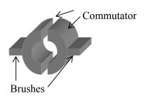
A loop with a commutator placed in a magnetic field forms a simple **DC motor**.
