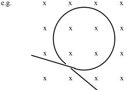
Pulling or pushing the two ends decreases or increases the area enclosed by the loop.
