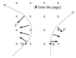
Use the **right-hand slap rule** to determine the direction of the magnetic force on the moving positive charge in the magnetic field. The magnetic force is always perpendicular to both the magnetic field and the direction of motion of the charge. If the positive charge is replaced by a negative charge, the force is in the opposite direction.
