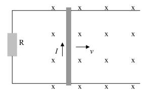
An external circuit of resistance R is connected to the conductor by two conducting rails on which the conductor slides along. A current *I* flows and a magnetic force opposes the motion. The conductor slows down to a stop when the generated electrical potential energy is expended.
