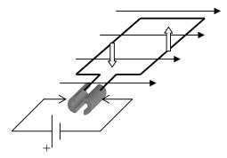
Example 1 A loudspeaker also works on the principle that a magnet exerts a force on a current-carrying wire.
