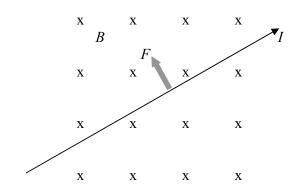
Again the direction of the magnetic force on the wire can be determined by using the right-hand slap rule. The magnetic force is always perpendicular to both the magnetic field and the current.
