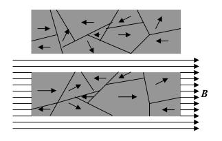
Example 1 Explain how a magnet can pick up unmagnetised iron nails and paper clips.
