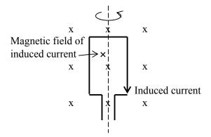
As the loop rotates from the orientation shown above the flux decreases because there are less magnetic field lines passing through the loop into the page. To *oppose* this the induced current flows clockwise (viewing the page) in order to generate more magnetic field into the page through the loop.
