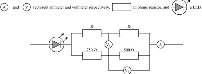
The meter readings are  $V_1 = 0$  volts,  $V_2 = 2.4$  volts and A = 10.8 milli-amperes.
