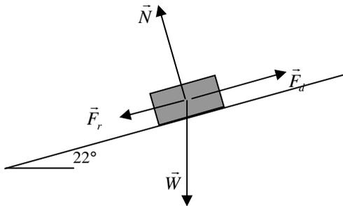
Since the car travels at constant velocity (zero acceleration),  $\therefore \vec{F}_{net} = \vec{F}_d + \vec{F}_r + \vec{W} + \vec{N} = \vec{0}$ , and therefore the component along the inclined plane (road) is zero. Choose uphill as the positive direction.
