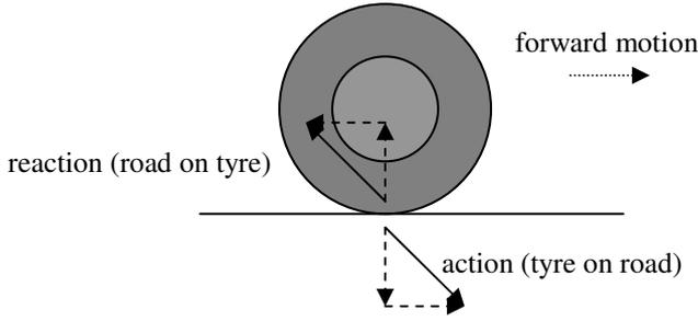
Force diagram showing the forces on the car (represented by the tyre) in *Newton's second law*:
