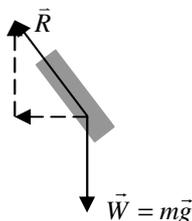
The net force on the cyclist is given by the horizontal component  $\vec{F}_f$  because  $\vec{W}$  and the vertical component of  $\vec{R}$  add to zero.
