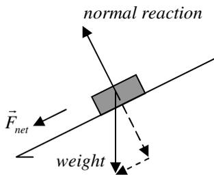
**Example 1** A 1200-kg car travels uphill at *constant velocity* along a road which inclines at an angle of  $22^\circ$  with the horizontal. Air resistance and rolling friction total 50 N oppose its motion. Analyse the forces acting on the car and determine the driving force.
