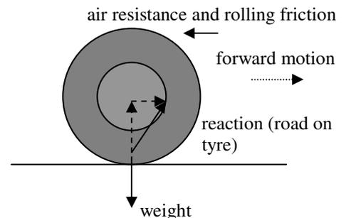
Example 4 A car slows down on a horizontal road whilst brakes are applied. Analyse the forces in Newton's third law between the tyres and the road surface. Analyse the forces in Newton's second law in relation to the motion of the car.
