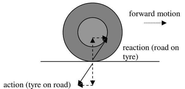
The reaction force has two components: the force of friction and the normal reaction of the road on the tyre.
