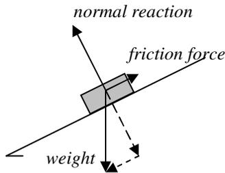
If there is no friction (or very little friction), the vector sum of the normal reaction force and weight, (the net force) is not zero, and the object slides down the slope with increasing speed.
