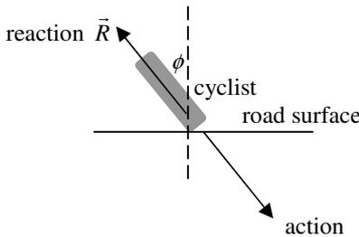
This reaction force  $\vec{R}$  has two components. The vertical component is the normal reaction force  $\vec{N}$ , and the horizontal component is the force of friction  $\vec{F}_f$ .
