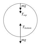
lnet force on the ball at the topl = lnet force on the ball at the bottoml
