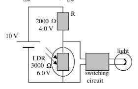
When the light intensity falls below 2.5 lux,  $R_{LDR} > 3000 \Omega$ .:  $V_{LDR} > 6.0 \text{ V}$  and triggers the switching circuit to turn on the
