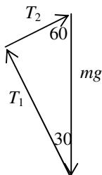
$$\frac{T_2}{T_1} = \tan 30, \therefore T_2 = \frac{T_1}{\sqrt{3}}$$
