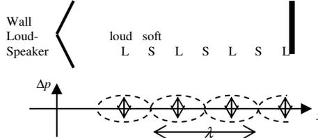
Every object has its own natural frequencies of vibration. If an energy source at one of these frequencies interacts with the object, the latter will be forced into vibration, a standing wave is formed. The object is in **resonance**. The natural frequencies of vibration are called **resonant frequencies**.
