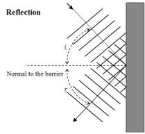
Wavelength, frequency and speed remain the same after reflection. Angles of incidence and reflection are equal,  $\angle i = \angle r$ . This is known as the **law of reflection**.
