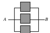
**Power in series and parallel circuits:** Total power consumption in parallel or series connection is the sum of the individual power of the components.
