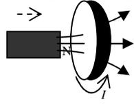
when magnet moves closer to the loop, magnetic field increases and the induced current  $I$  is as shown.
