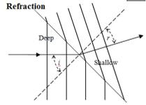
The wave changes its speed and direction when the depth of water changes. Frequency is the same in both regions.
