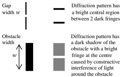
Extent of diffraction  $\propto \frac{\lambda}{w}$ . Significant effect when  $\frac{\lambda}{w} \approx 1$ .
