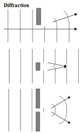
Wavelength, frequency and speed remain the same after diffraction. Spread due to diffraction
