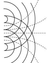
The diagram (left) is called an **interference pattern** of two circular waves generated by two sources producing the waves periodically and **in phase**. Wavelength, frequency and speed remain the same during and after interference.
