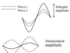
Two waves interfere when they cross or overlap each other. If they are in phase (crests meeting crests and troughs meeting trough), **constructive interference** is said to occur resulting in a wave with larger amplitude.
