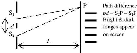
Constructive interference (bright):  $pd = 0\lambda, 1\lambda, 2\lambda, \dots$
