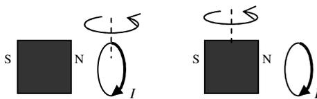
Direction of induced current and polarity of output terminals of a generator are determined by **Lenz's Law**: an induced current in a conducting loop flows in a direction such that the magnetic field of the induced current *opposes* the change in magnetic flux that produces it. The terminal that the induced current flows to is +, the other -.
