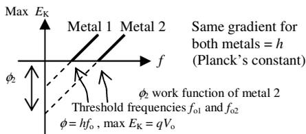
Failure of the wave model to explain the photoelectric effect
