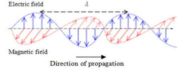
**Polarisation of light** Light emitted by an excited atom is polarised, i.e. the oscillating electric field lies on the same plane along the direction of propagation. Polarisation of light is a good indicator that light as a wave is transverse.
