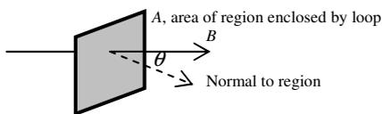
**Electromagnetic induction** is the generation of electricity by changing magnetic flux. The generated current is called **induced current  $I$** ; the generated voltage is called **induced emf  $\xi$** .
