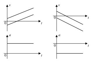
The gradient of a velocity-time graph gives the acceleration, and the area 'under' an acceleration-time graph gives the change in velocity (not velocity).
