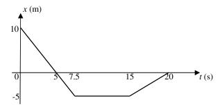
Initially, the object is 10 m east of the origin. It travels 15 m to the west in 7.5 s. Now it is 5 m west of the origin and remains there for another 7.5 s before it turns around and travels 5 m to the east in 5 s, finishing at the origin. Its displacement in the 20 s is -10 m, and the total distance travelled is 20 m.
