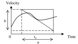
Acceleration (at  $t = t_0$ ) = gradient of tangent =  $-\frac{b}{a}$
