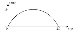
The object starts from the ground and moves vertically upwards to a maximum height of 4.9 m in 1.0 s and falls back to the ground in another 1.0 s. The displacement in the 2.0 s is 0 and the total distance travelled is 9.8 m.
