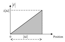
The area of the shaded region gives the work done in compressing or extending the spring by  $|\Delta \vec{x}|$ .
