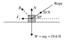
Note: Reaction force  $\vec{R}$  is resolved into  $\vec{N}$  and  $\vec{F}_f$  in the diagram.
