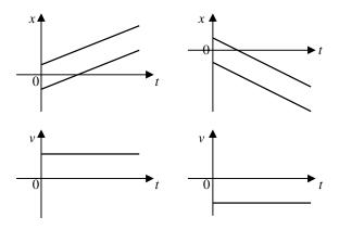
Gradient of a position-time graph gives velocity, and area 'under' a velocity-time graph gives displacement (not position).
