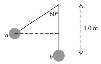
From a to b the distance fallen =  $1.0-1.0\cos 60^{\circ} = 0.5$  m.  $mgh_a + \frac{1}{2}mv_a^2 = mgh_b + \frac{1}{2}mv_b^2$ ,  $m(9.8)(0.5) = \frac{1}{2}mv_b^2$ ,  $v_b \approx 3.1 \,\text{ms}^{-1}$ .
